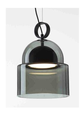
Tech. description The luminaire consists of a glass shade, metal frame with integrated LED module, metal printout on the lower edge of the screen, supply cable and steel cable. The luminaire is suspended from the ceiling canopy by means of a supporting steel cable.
